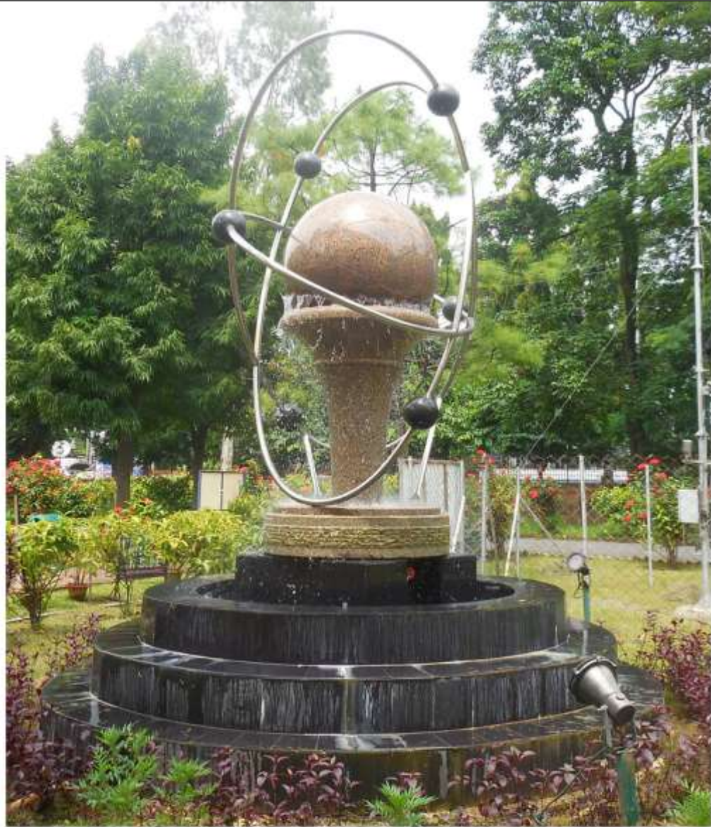
Granite Ball Ellipse Fountain Granite Ball Diameter = 1 metre and Weight = 1 ton Three 38 mm diameter S.S. pipe Ellipses with 3 meter major axis & 1.7 meter minor axis.
